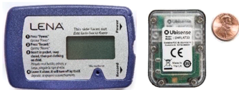
Fig. 2. LENA Digital Language Processor and Ubisense tag. Note: The LENA Digital Language Processor measures 2.2" x 3.4" x 0.5". The Ubisense tag measures 1" x 1" x 0.36". Photos courtesy Laura Vitale.
